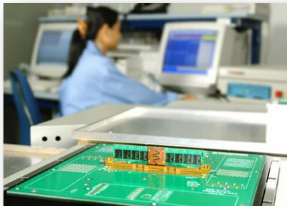
Checking early FB-DIMM prototype against specifications
