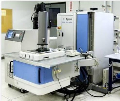
DDR4 DRAM chip validation testing on new Advantest tester
